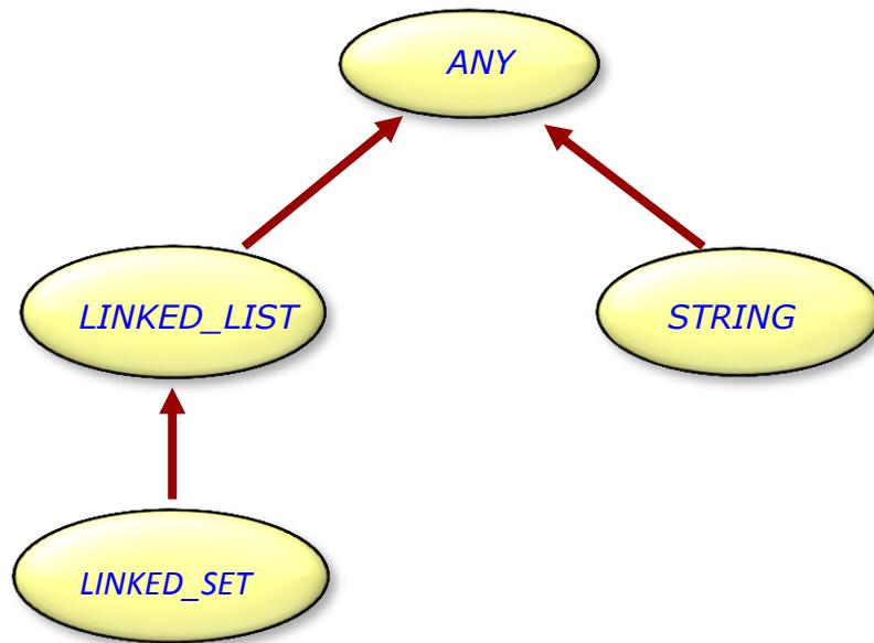
The reusable visitor pattern associates an agent for each type. That is: process\_any for type ANY; process\_list for type LINKED\_LIST; process\_set for type LINKED\_SET and process\_string for type STRING. When an item is to be processed, the visitor traverses the type conformance hierarchy until it finds an agent suitable for that item.
