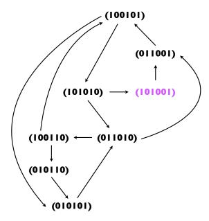
The buffer is never both full and empty because the graph contains no marking with  $M(\text{buffer\_empty}) = M(\text{buffer\_full}) = 1$ .
