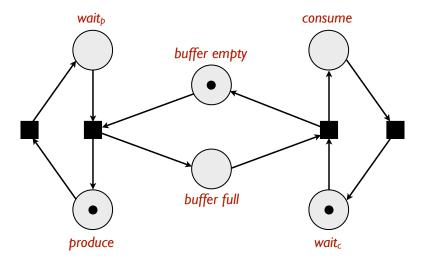
Construct a reachability graph for the Petri net, and prove that the buffer is never both full and empty.
