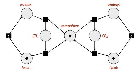
For each process i add a place noncritical<sub>i</sub> that holds a token if and only if that process i is not in its critical region.
