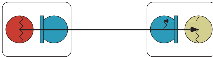
Figure 2.2: Message Passing Interaction with an Unconnected Socket
