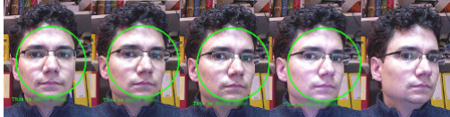
Figure 3. Face detection and recognition. Only the frontal face and slightly turned faces are detected. The text below the green circle indicates recognition of the detected face.
