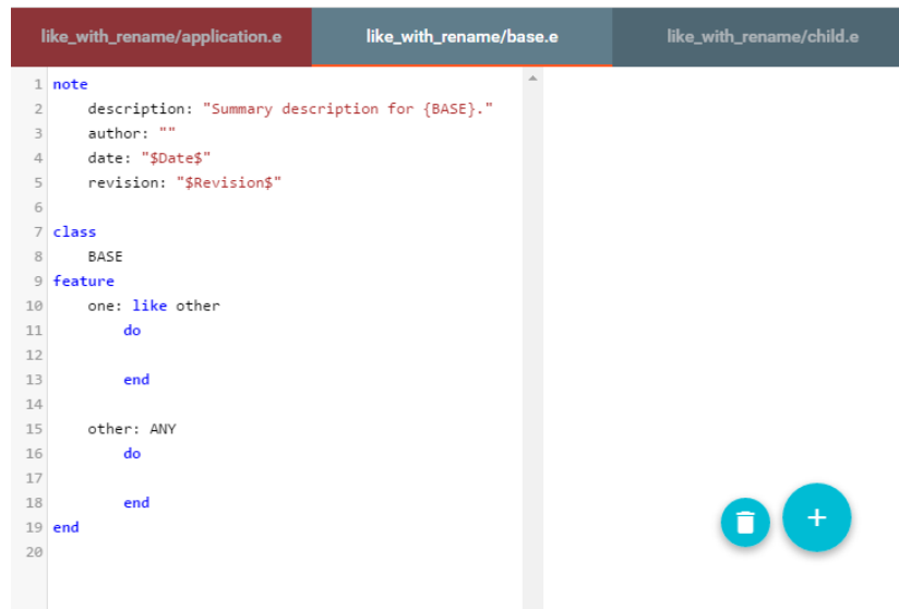
Figure 4.4: Tabbed interface with error indicator and new & delete file buttons
