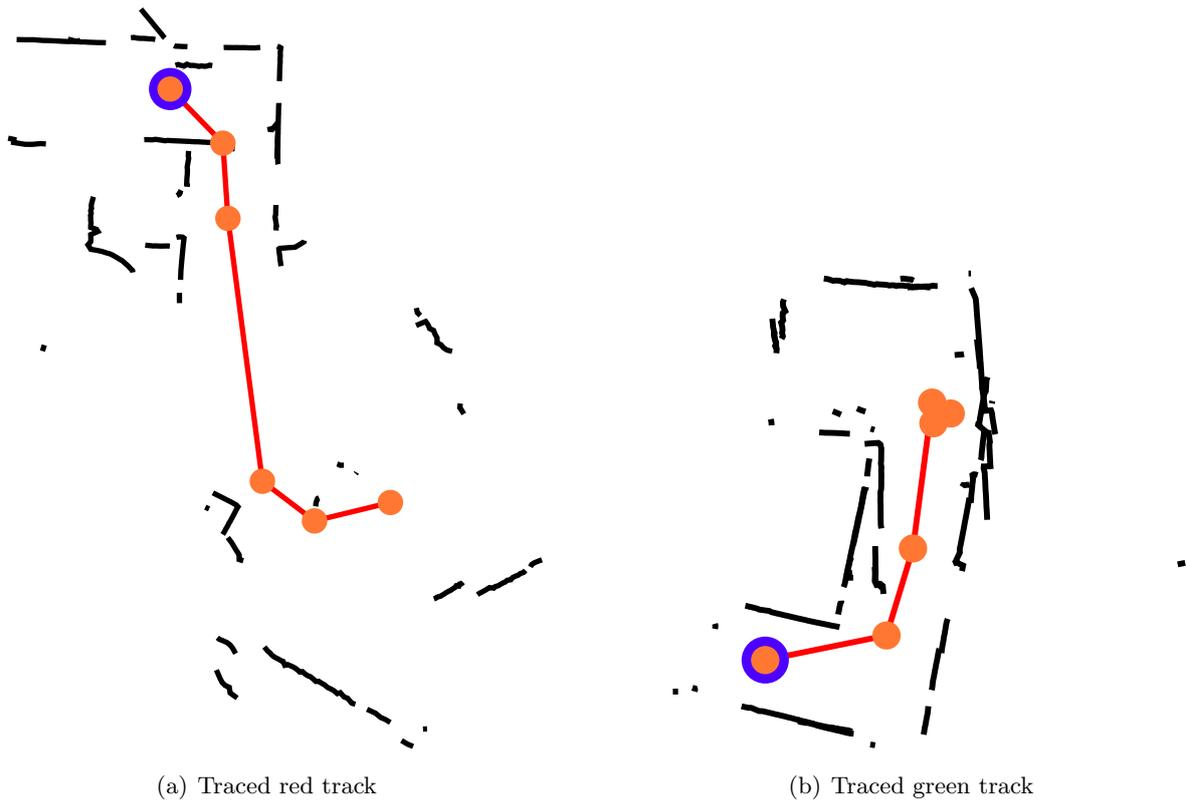
Figure 25: Traced environment with CSM algorithm
