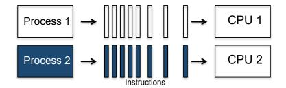
Figure 1: Multiprocessing: instructions are executed in parallel
