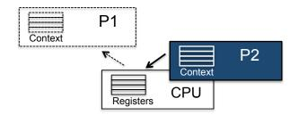
Figure 3: Context switch: process P1 is removed from the CPU and P2 is assigned to it
