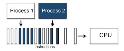
Figure 2: Multitasking: instructions are interleaved
