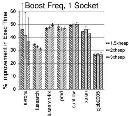
Figure 2. Percent execution time improvement when boosting frequency from lowest to highest on one socket.
