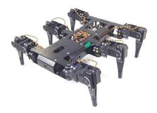
Fig. 8: The hexapod has six legs with three degrees of freedom.
