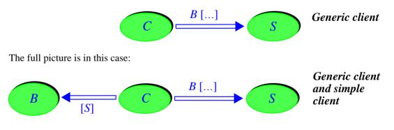
Do not confuse the two forms of client relation arising here: C is a simple client of B, with S as a generic parameter, through the declaration of x (left part of the figure); but that declaration also makes C a generic client of S, assumed here for simplicity to be a non-generic class..
